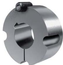
Taperlock clampings are the standardized, commercially available machine parts for creating non-positive shaft-to-hub connections with a pulley. The conically slotted bushing with feather key groove according to DIN 6885 serves to fasten pulleys to shafts or journals.
