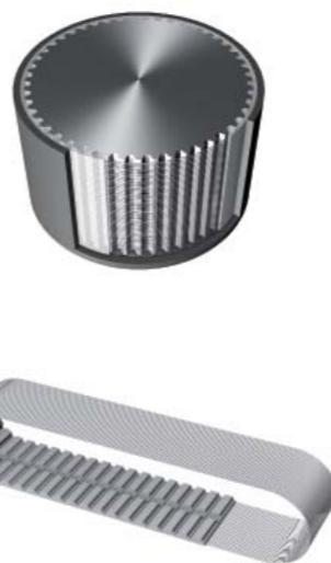
**Polyurethane molded timing belts** (sleeves) are cast in special molds. These types of belts feature very exact pitch sizes along the whole belt and are particularly suitable whenever smooth running and high-speed drive are needed.
