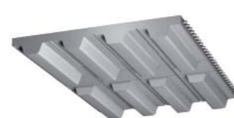
**easy drive® polyurethane timing belts "Flex"** are extruded with endless wound cords. In these belts the cords are helically spooled. Due to the high power transmission capacity of these belts, they can be used universally for power transmission as well as conveying and positioning applications.
